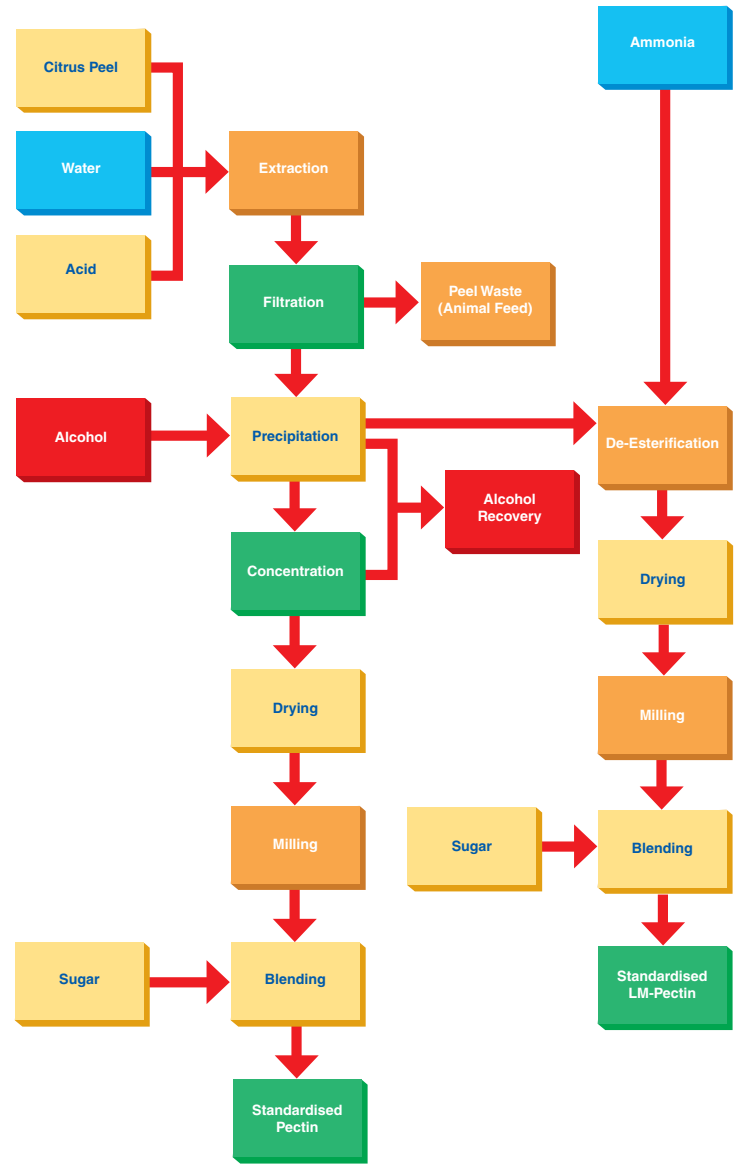
Figure 2. Flow Chart: Production of Pectin
